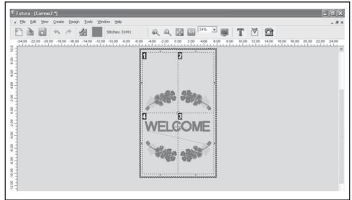
4. The design data is sent to the machine for sewing one section at a time. Click on the “Transmit to Machine” tool on the tool bar.
